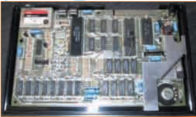
Inside the rubber-keyed Spectrum. Note the internal speaker in the bottom-right corner
